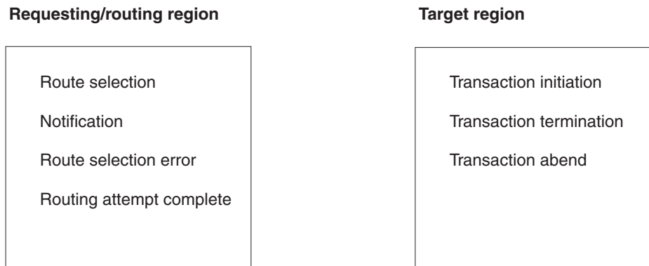
Figure 70. When and where the distributed routing program is invoked
