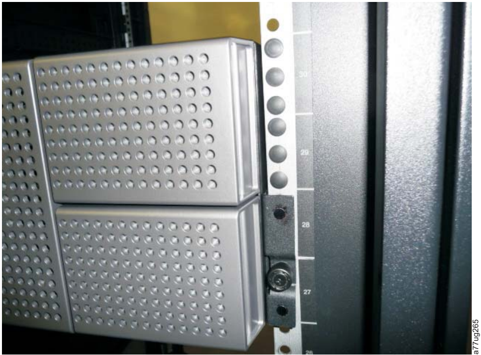
Figure 4-14. Securing the 2U library to the rack
