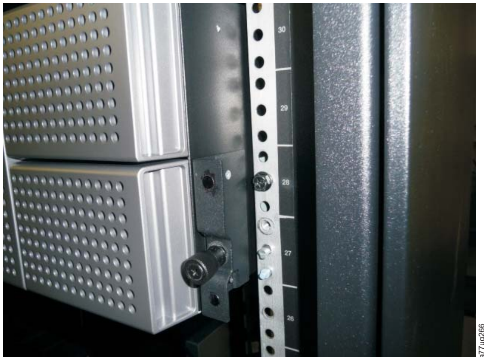
Figure 4-13. Sliding the 4U library into the rack
