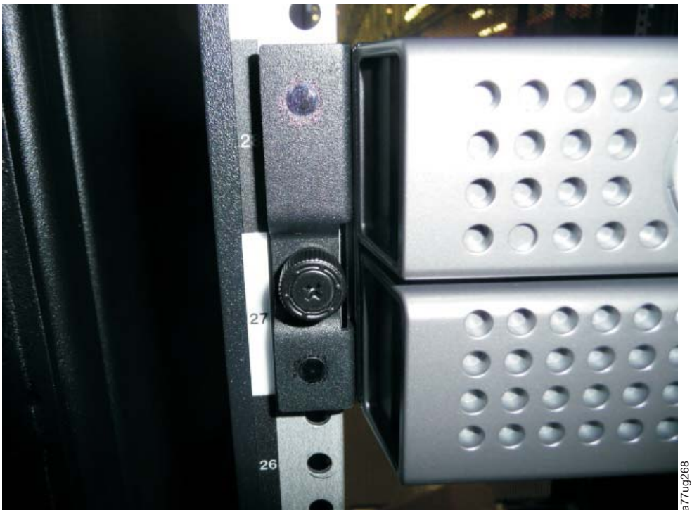
Figure 4-15. Securing the 4U library to the rack
