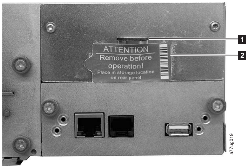
Figure 4-3. Library shipping lock and label storage location
