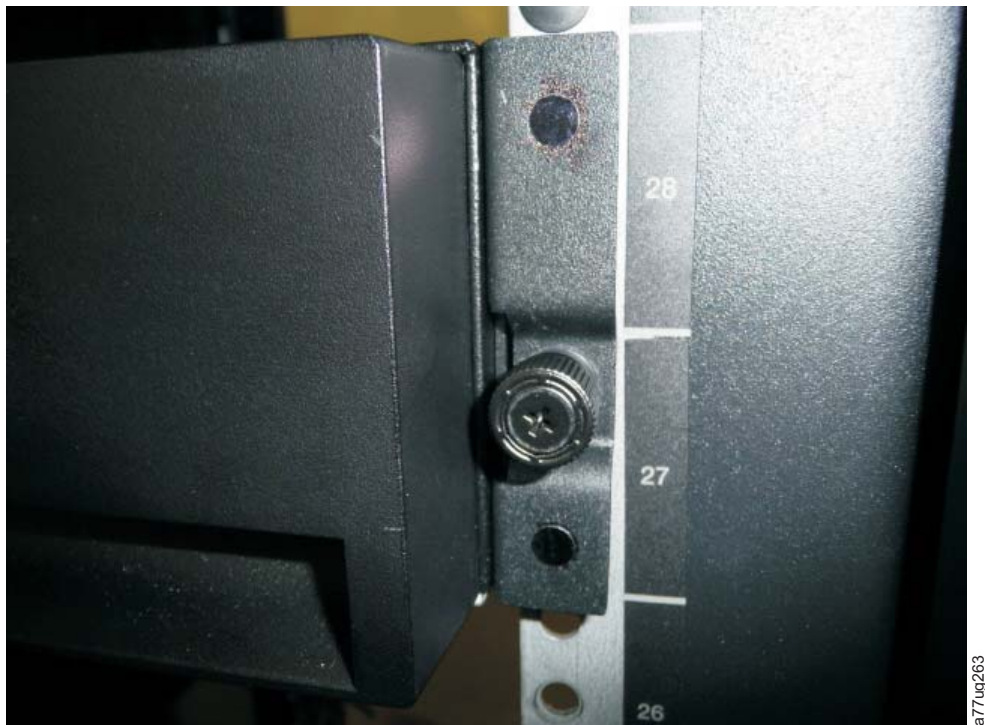
Figure 4-10. 2U library side screws to remove
