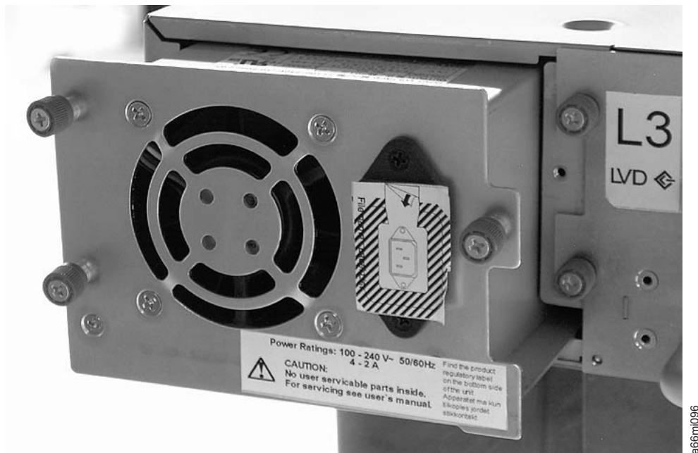
Figure 10-21. A power supply being removed from a library
