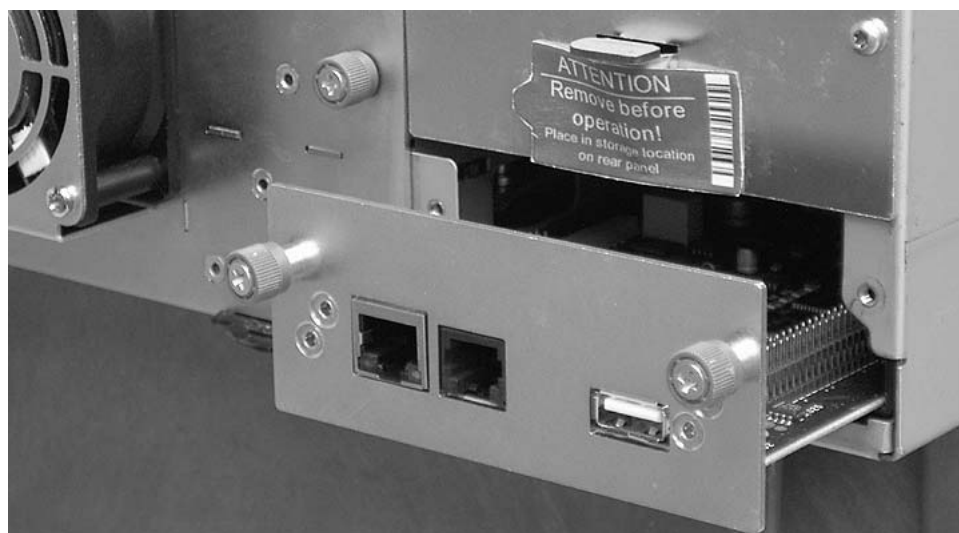
Figure 10-22. Removing a Library Controller Card from the library
