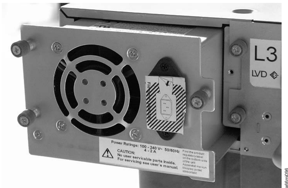
Figure 10-12. A power supply being removed from a 2U library
