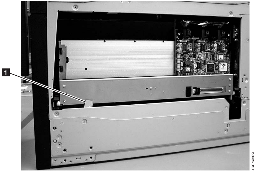
Figure 4-18. Bottom view of picker assembly lock mechanism
