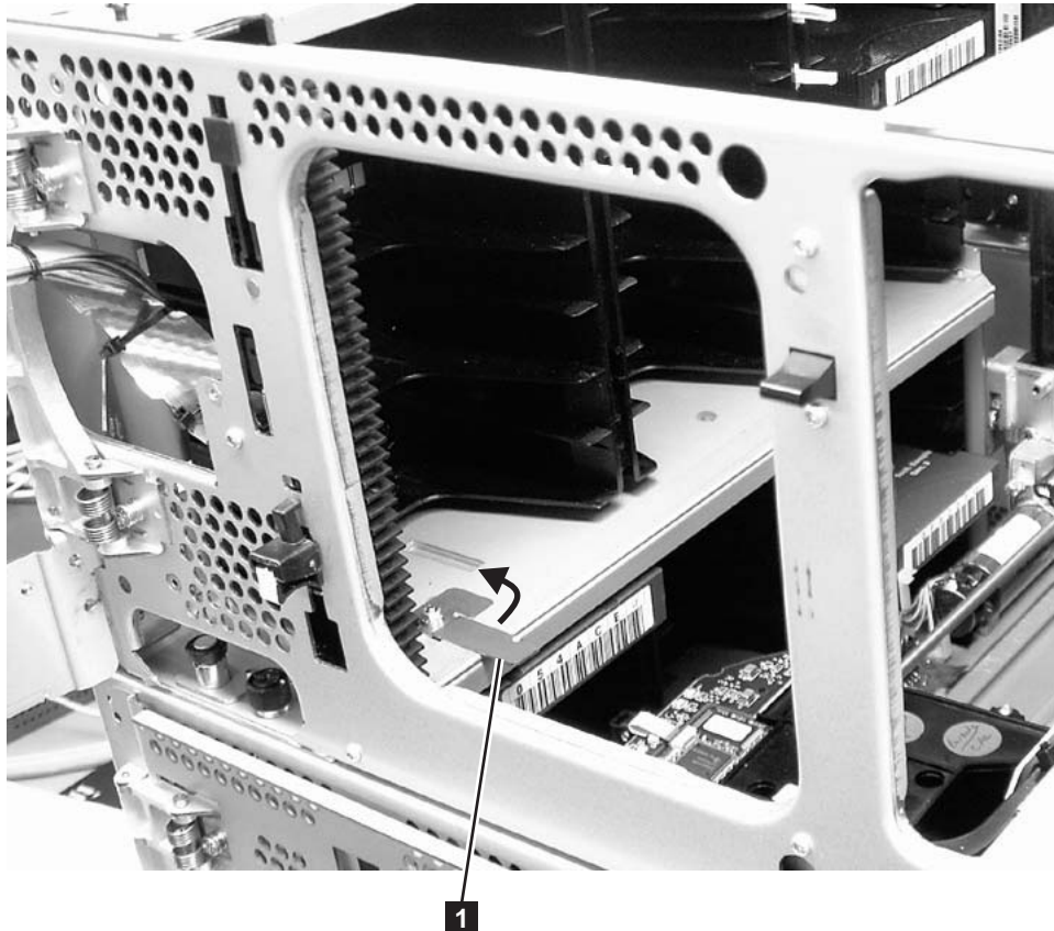
Figure 4-30. Releasing the picker assembly lock mechanism
