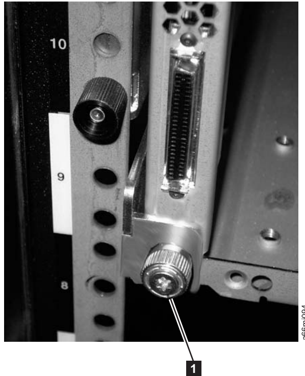
Figure 3-24. Rear flange and thumb screw on rack rail
