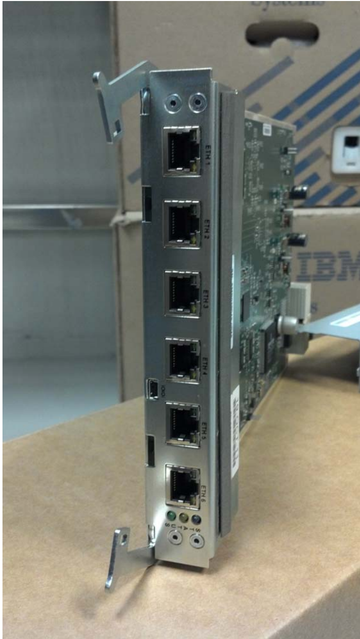
Figure 12-41. Ethernet Expansion Blade - installation
