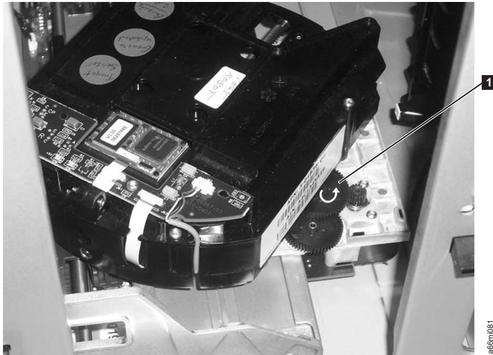
Figure 10-10. Picker that is rotated for drive gears access
