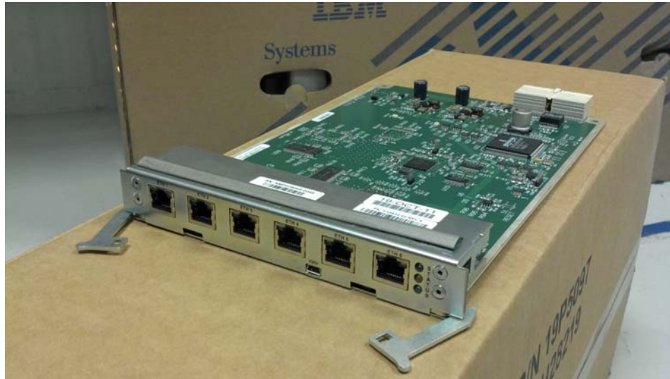
Figure 12-40. Ethernet Expansion Blade - horizontal view
