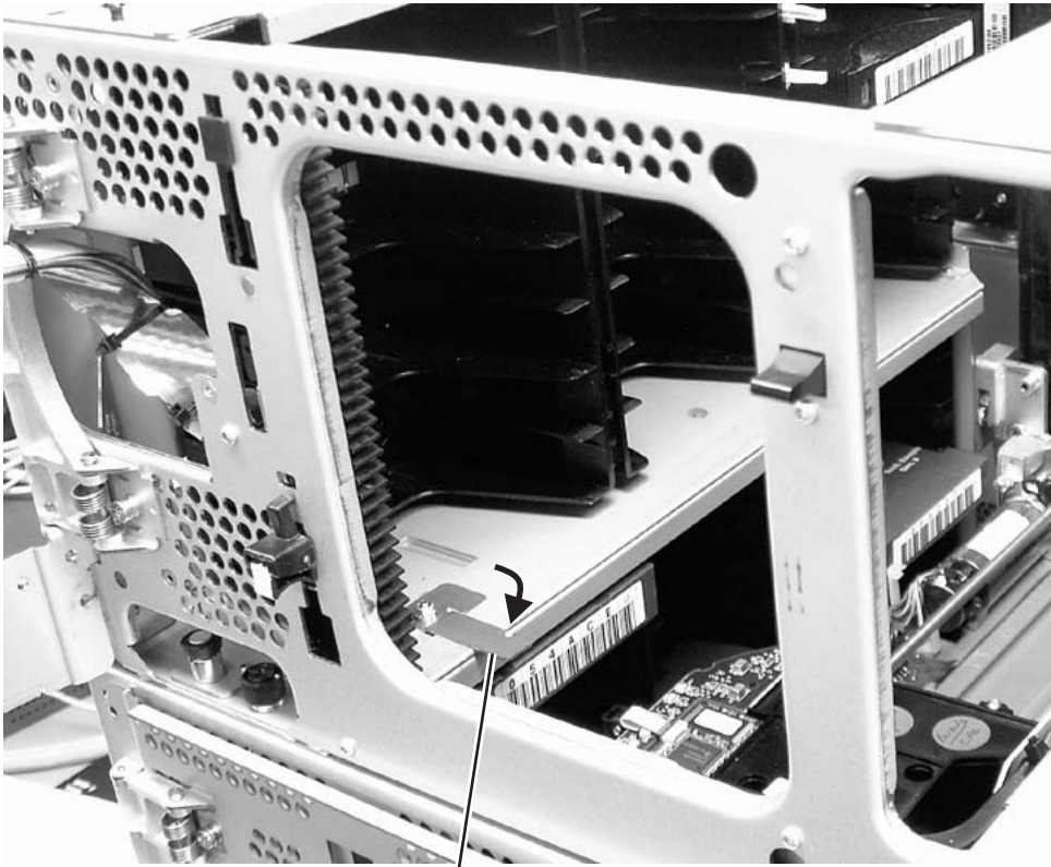
Figure 3-25. Picker assembly lock mechanism
