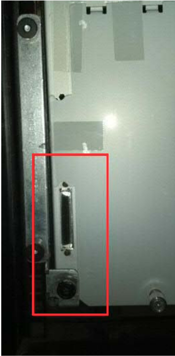
Figure 12-39. Module Communication Terminator is removed
