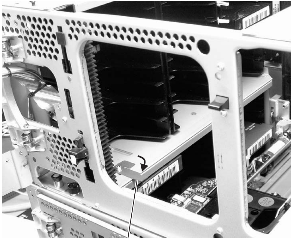
Figure 12-20. Picker assembly locking mechanism
