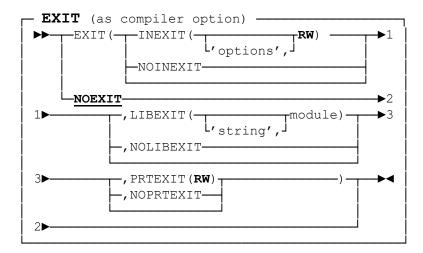
This is the option that enables the precompiler to run under the control of the compiler. Abbreviations are: **EX**, **INX**, **LIBX**, **PRTX**.
