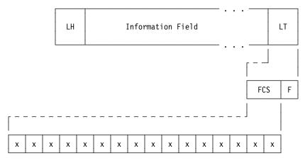
Figure 1-8. Frame Check Sequence Field of Link Trailer
