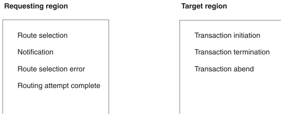
Figure 72. When and where the distributed routing program is invoked
