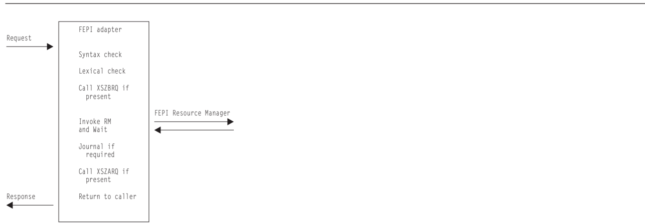
Figure 53. Logic flow within the FEPI adapter
