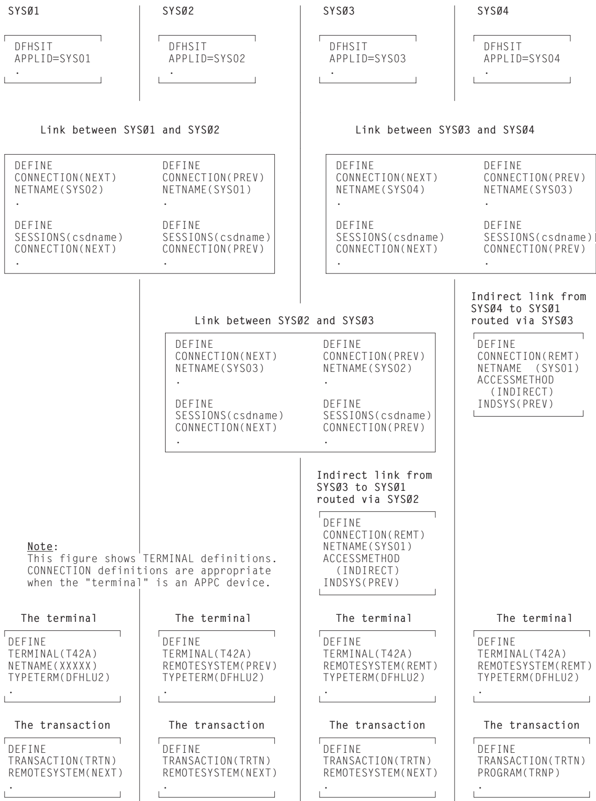
Figure 50. Defining indirect links for transaction routing. Because the remote terminal definitions in SYS04 and SYS03 do not specify the REMOTESYSNET option, indirect links are required.
