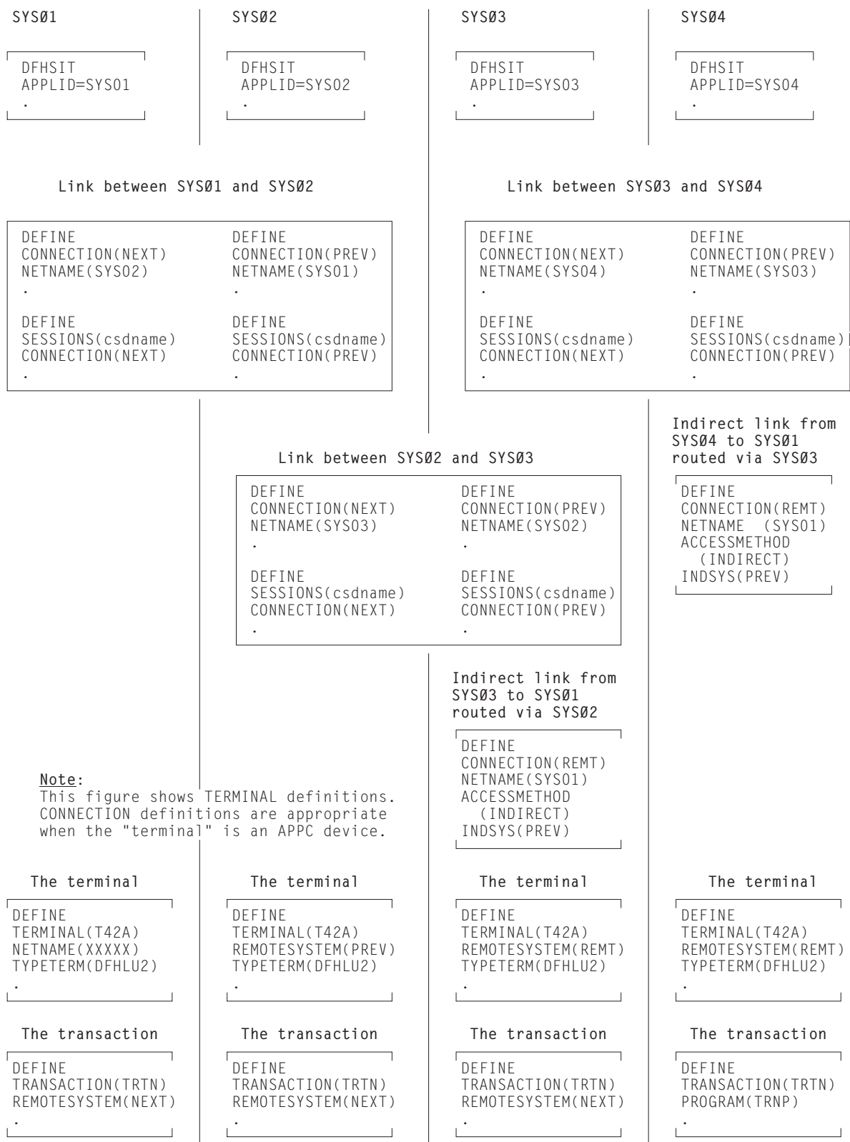
Figure 55. Defining indirect links for transaction routing. Because the remote terminal definitions in SYS04 and SYS03 do not specify the REMOTESYSNET option, indirect links are required.
