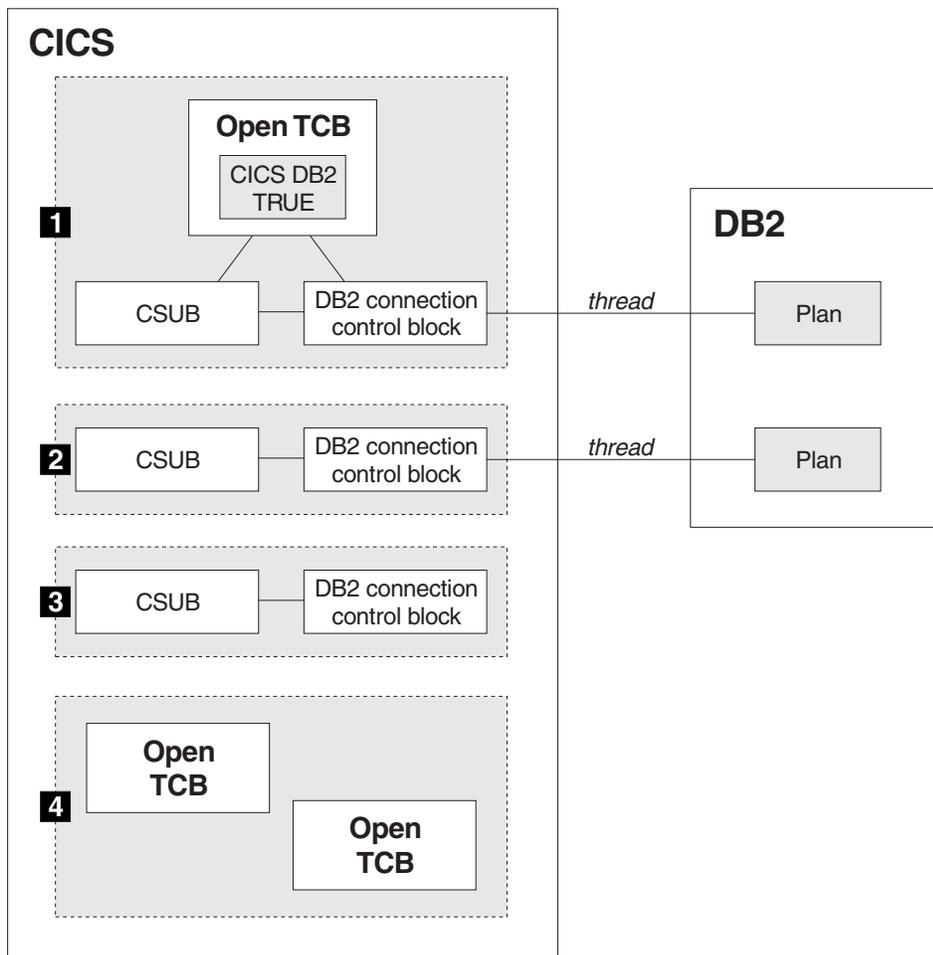
Figure 2. Thread TCBs in the open transaction environment
