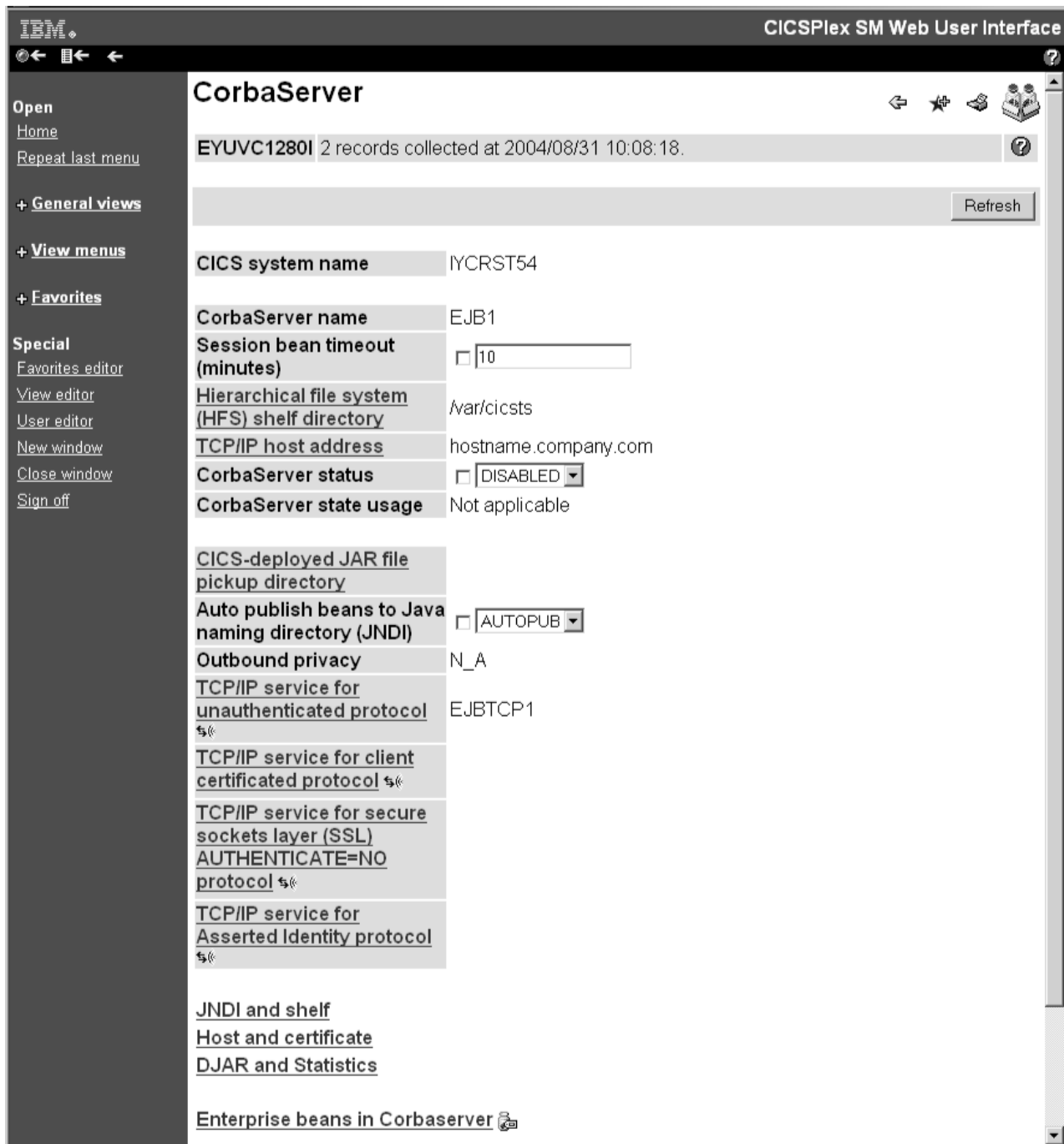
Figure 10. Detail of the CorbaServer EJB1
