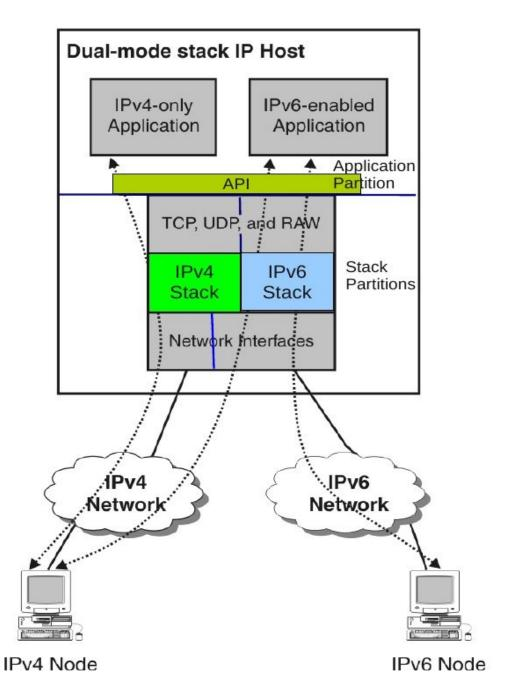
The above diagram shows the basic layout of a dual stack system. When an API call is made the stack ID used determine the stack to be used. Based on the type of stack either the IPv4 or the IPv6 API routines are entered.
