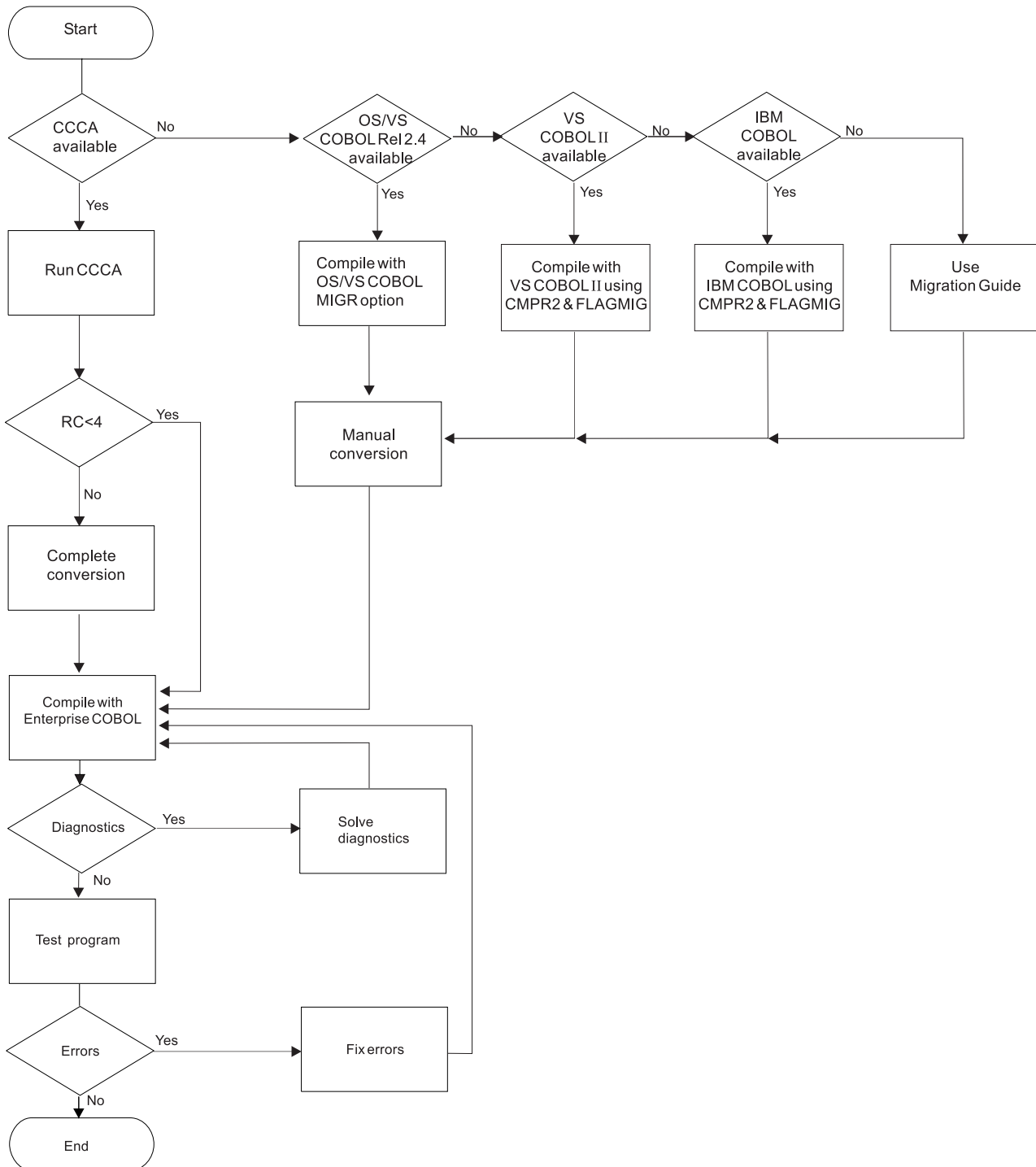
Figure 1. Steps for converting an OS/VS COBOL program to an Enterprise COBOL program
