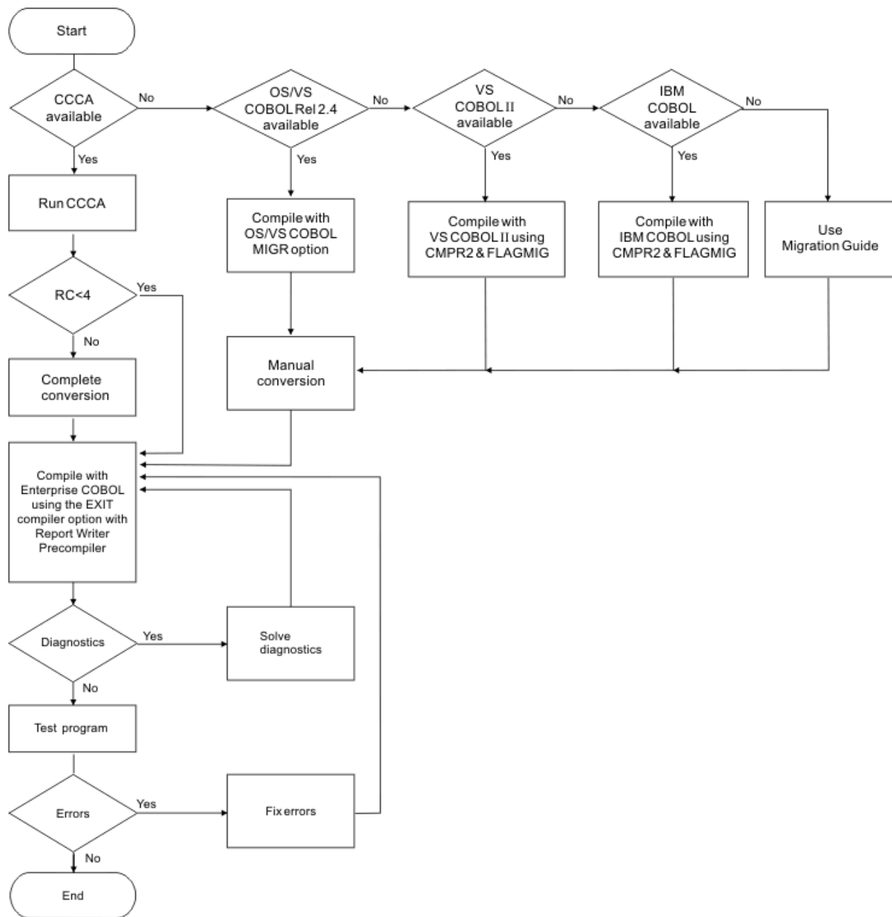
Figure 4. Steps for converting an OS/VS COBOL program and retaining Report Writer statements
